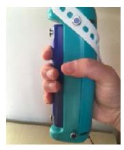
The straps have a small element of stretch in them to aid fixation but it is important that the straps are not fixed too tight. Consider the route of the superficial branch of the radial nerve and be sure not to compress in this area. Wherever possible, use the hooks that are on the main body of GripAble rather than the two on the moveable fingerplate. If the latter hooks are needed, GripAble should be used in the isometric mode (see below).
